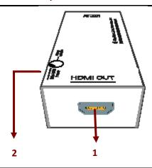
1. HDMI OUT 2. Mini USB & 5V DC Power Connector
