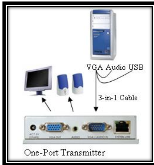
Installation Diagram of System Transmitter VGA-C5-S
