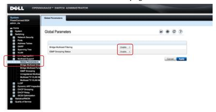
3. Go to Switching ---> Multicast Support ---> IGMP Snooping ---> set IGMP Snooping Statu to Enable, set IGMP Querier Status to enable
