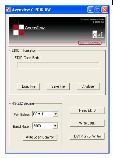
Ensure that power is connected and proper Com Port is selected. Then click on Auto Scan ComPort
