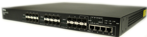
FIBER Network Switch with copper ports
