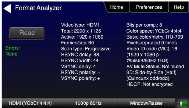
**Figure 11: 780A Format Analyzer Test Screen**
