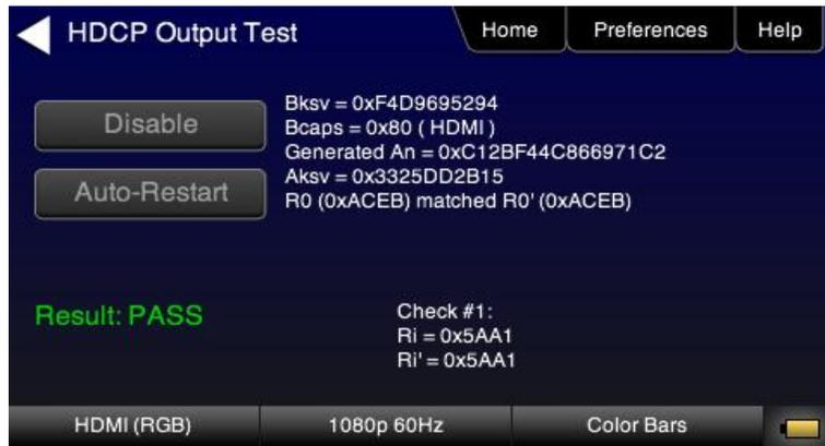
**Figure 5: 780A HDCP Functional Test**
