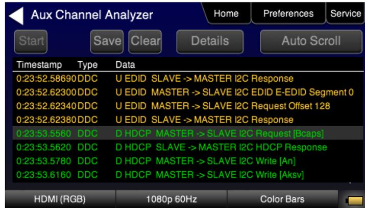
**Figure 14: 780A Screen showing DDC transactions logged**
