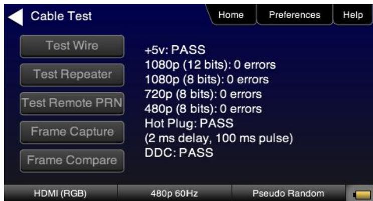
**Figure 4: Cable and Repeater Loop Test Results Screen**
