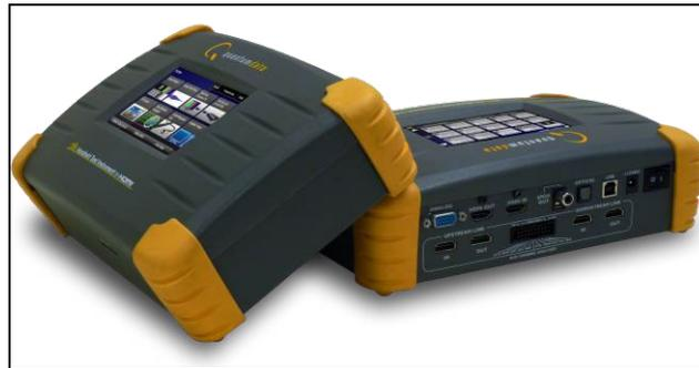
**Figure 2: Quantum Data 780A Test Instrument**
