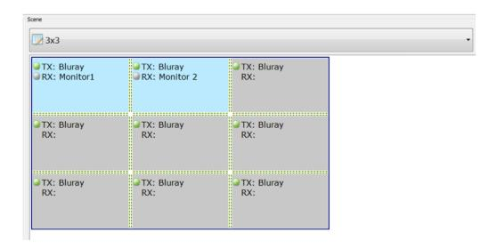
STEP 6: The user can easily right click on the Videowall created and choose Change TX, this will allow simple switching of any of the searched TX in the listed devices to be displayed across the Videowall.
