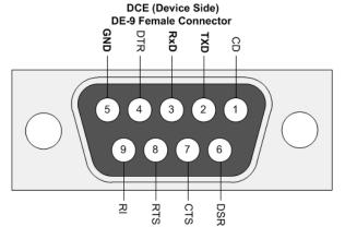
**RS-232 Connector Pinout**
