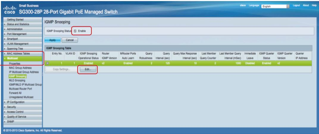
3. In Multicast > IGMP Snooping select VLAN the switch is attached to and press Edit > Enable IGMP Snooping Status, Enable IGMP Querier Status, Select IGMP Querier Version IGMPV2
