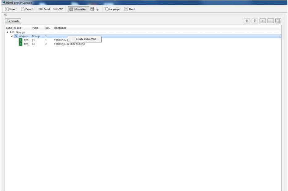
Step:3. In **Group I** create a 2x2 video wall **Zone I Scene2** with two rows and two columns.
