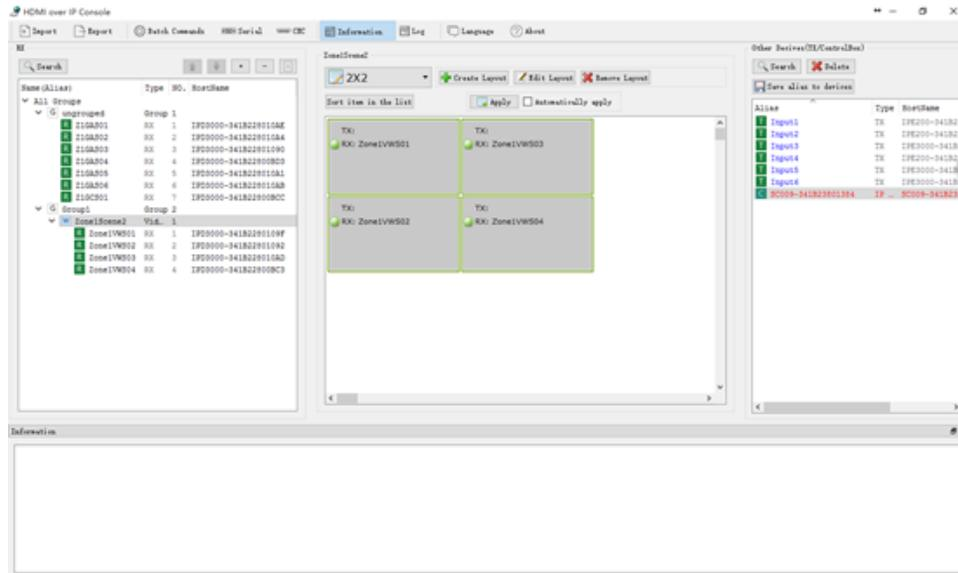
2) Select the four screens by right clicking on the screen on the upper left corner and moving the cursor while holding the right mouse until all four screens are highlighted. In the displayed context menu, choose **Combine**.
