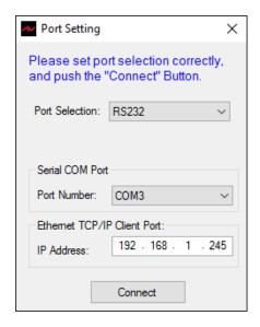
Once connection between the computer and the DVI-SPLITPRO-2X is established, the Control Interface will be displayed.
