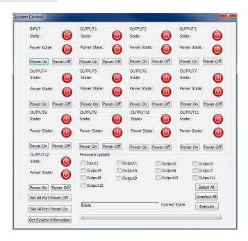
This tab has been made available because of the new DVI Modular PCB card design. This allows the user to add /remove Modular cards to the unit up to 12 Output cards, and configure and update their status individually;
