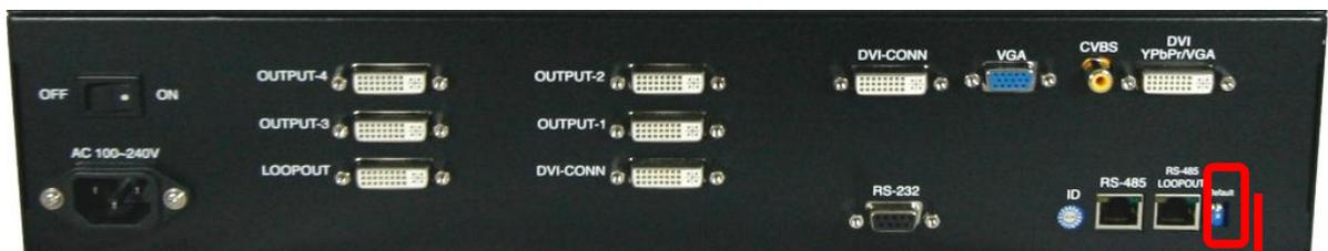
*To reset the DVI-VIDEOWALL-4 to factory default settings: Turn on the DVI-VIDEOWALL-4 then switch both DIP Switches simultaneously up and down to reset the unit to factory default settings*
