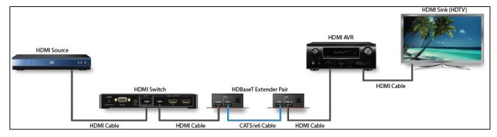
Figure 1: Typical HDMI Distribution Network with HDBaseT Extender
