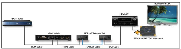
Figure 7: 780A End to End Frame Compare Test Configuration
