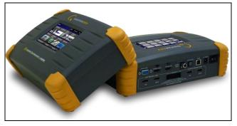
Figure 2: Quantum Data 780A Test Instrument Supports 4K capable HDMI devices at pixel rates up to 297MHz!
