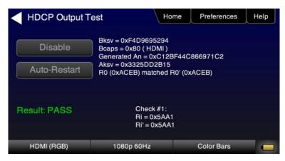
Figure 5: 780A HDCP Functional Test
