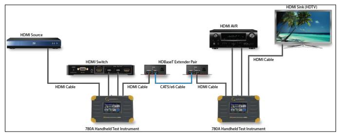
Figure 13: 780A Passive Monitoring of DDC traffic
