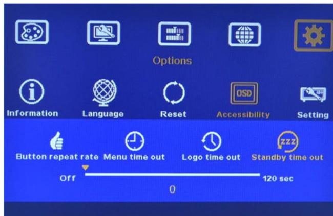
The default setting for [Standby Time Out] is 60 seconds. MLT-PROWALL-4K will automatically cut off output signal if no input signal is detected after 60 seconds. The time can be set by user. If the time is set to "0", then MLT-PROWALL-4K will not turn off the output signal even no input signal is detected.
