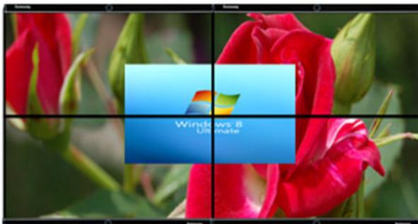
POP: to select POP (Picture outside Picture) display mode. User can select maintain original image aspect ratio or full screen mode through [Scaling] OSD menu under [Image properties]. If user set the system through Dip SW, user can select [POP Raw] and [POP Full] directly from front panel.
