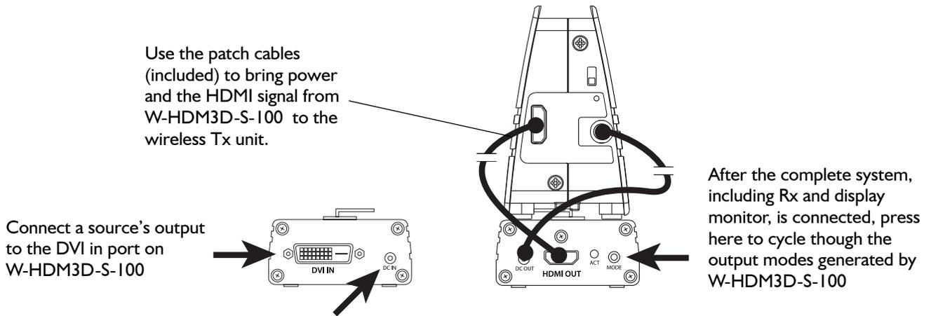
Connect the power cord into an available electrical outlet, and to the DC in port on W-HDM3D-S-100 . As with the Rx and Tx units, the DC Splitter accessory can be used to obtain power from an FSN medical display monitor.
