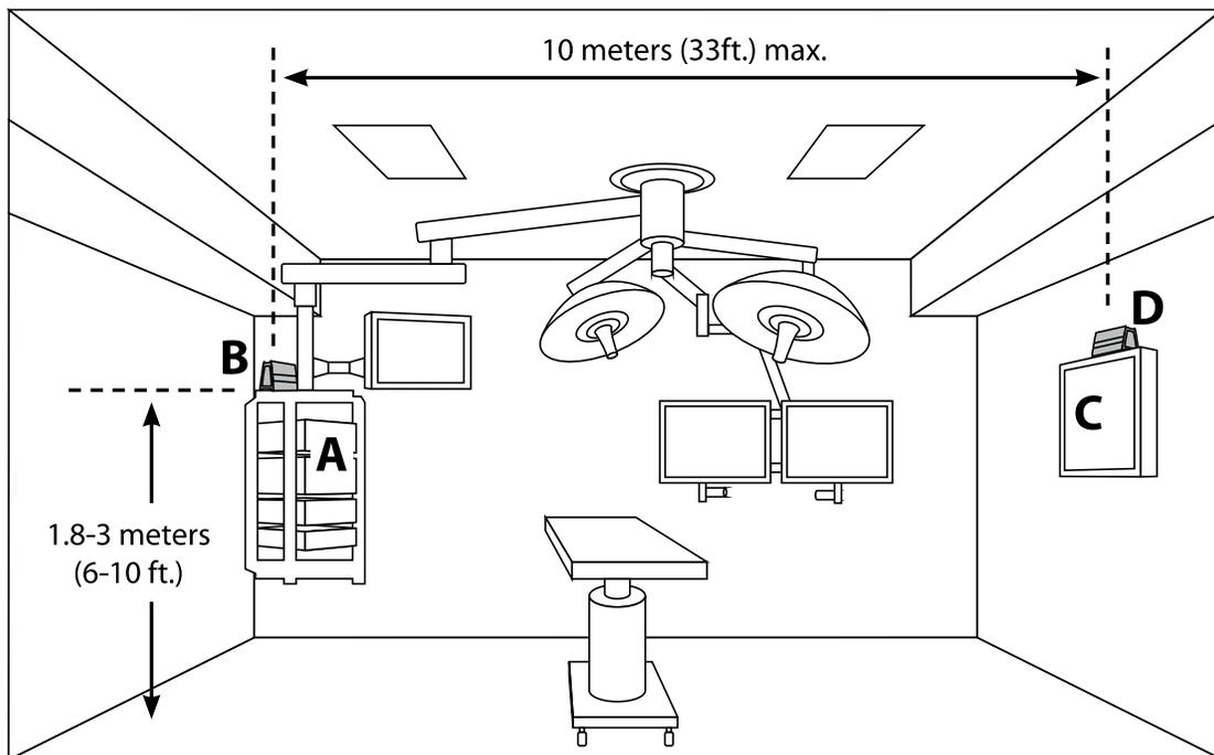
The transmitter and receiver units can stand alone on a flat surface, or use various brackets to mount onto other objects such as a display monitor. It is recommended to verify that the wireless system is operating properly before mounting the Tx or Rx units permanently. See the W-HDM3D-S-100 user guide for complete mounting instructions.
